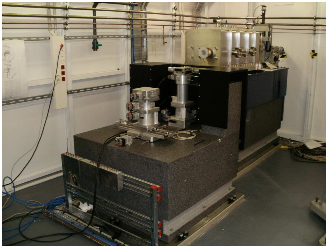
Figure 1. BL04-MSPD: High pressure towers of BL04-MSPD's high pressure End Station.
